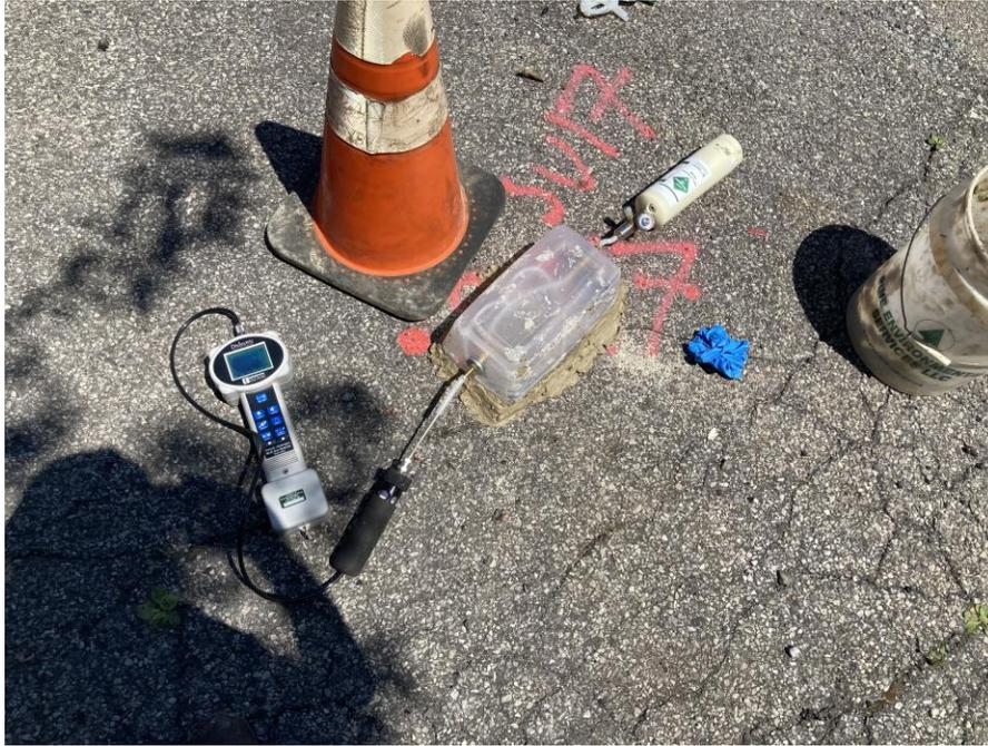
Photo 3: View of helium tracer test at SV-17
