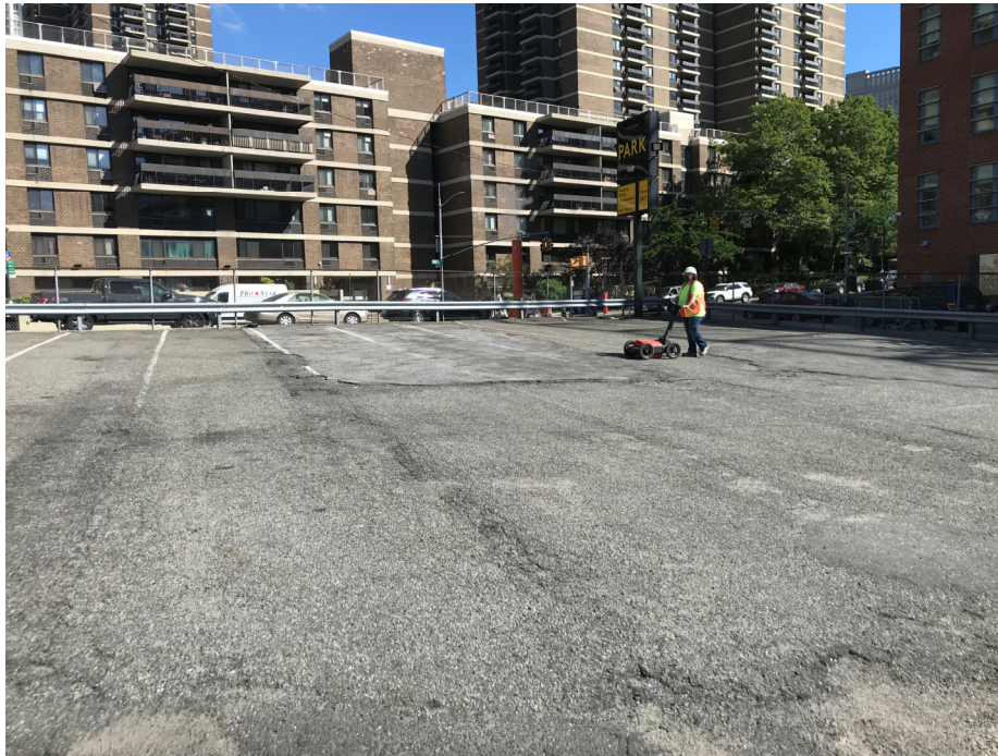
Photo 1: Hager-Richter using a GPR Scanner in the northern part of site (facing northwest)
