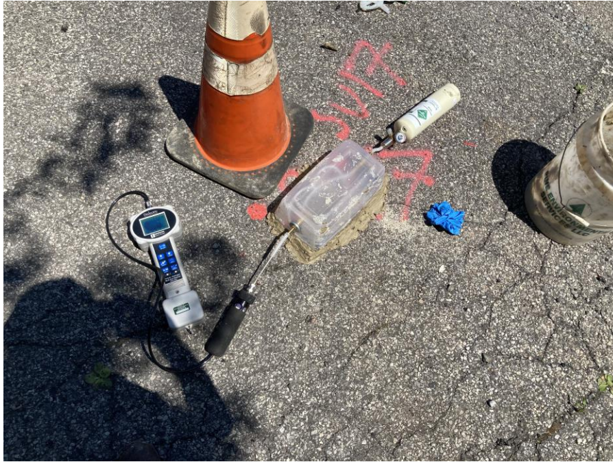
Photo 3: View of helium tracer test at SV-17
