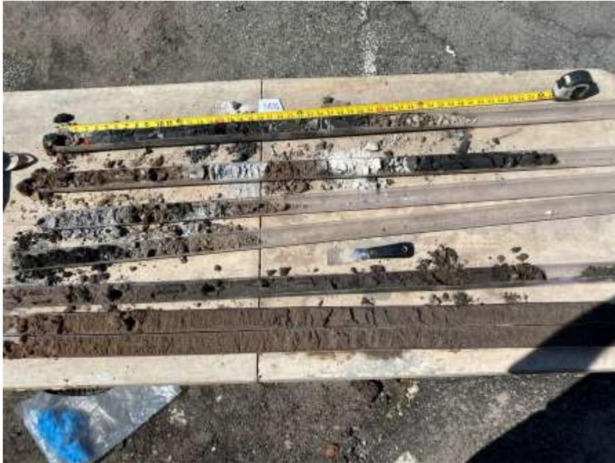
Photo 1: View of soil from boring SB36
