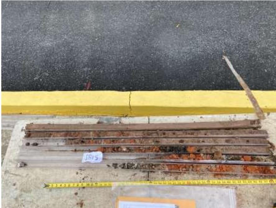
Photo 1: View of soil from boring SB15.
