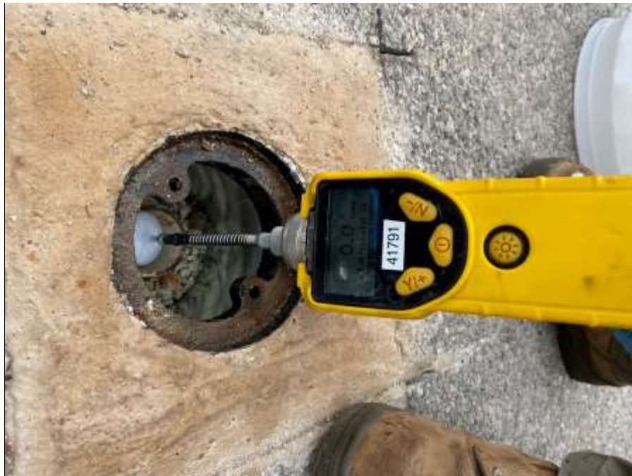
Photo 2: PID screening of monitoring well MW15
