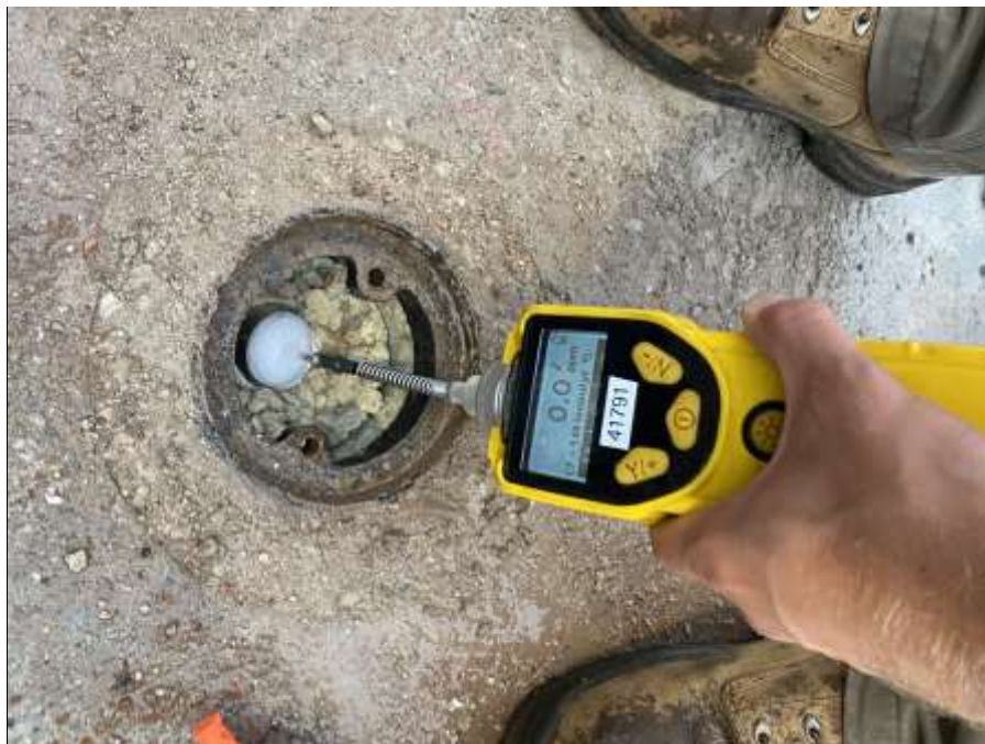
Photo 2: PID screening of monitoring well MW33
