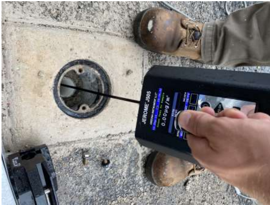
Photo 3: Jerome screening at monitoring well MW34
