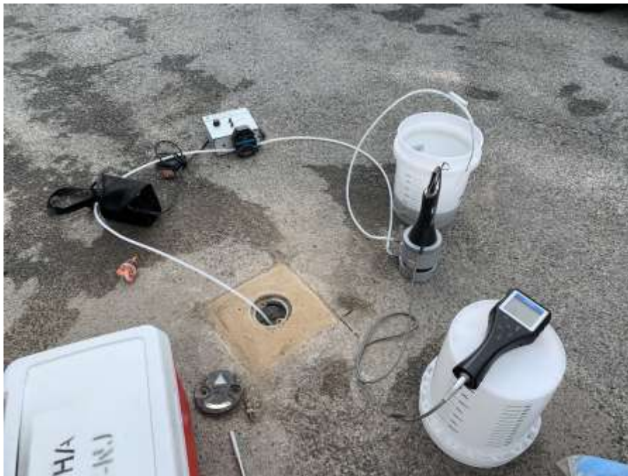
Photo 4: Typical groundwater sampling set up
