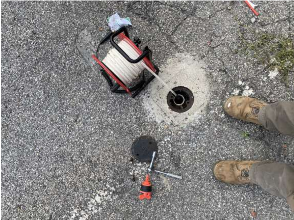
Photo 1: View of typical monitoring well gauging.
