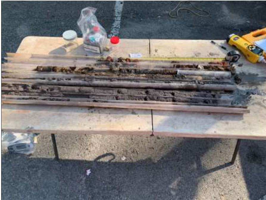
Photo 1: View of soil from boring SB35
