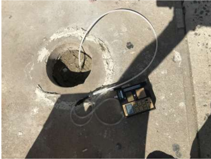
Photo 3: View of Langan collecting a mercury vapor sample at SV39 (facing south)
