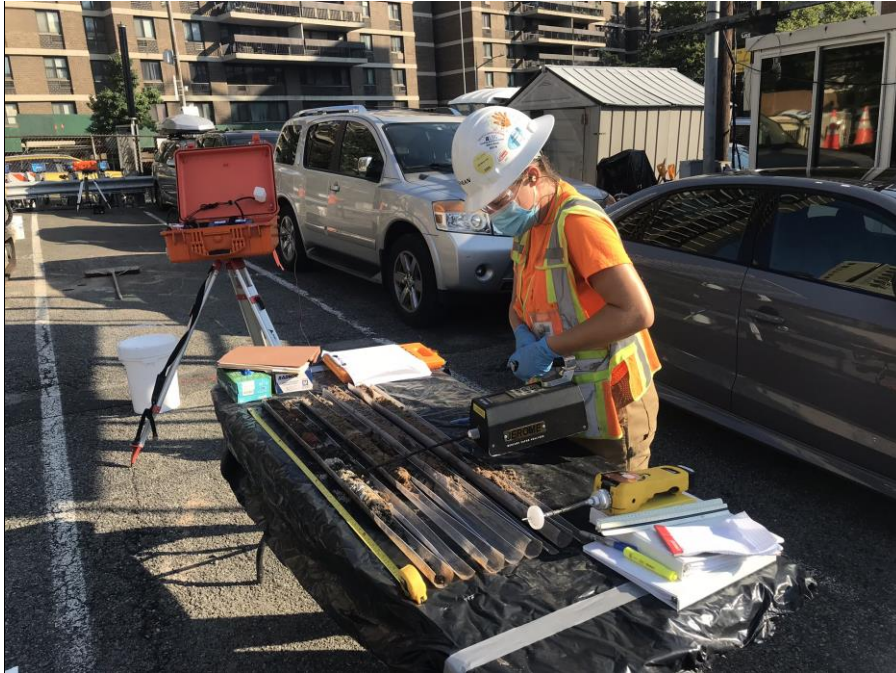
Photo 3: Langan collecting mercury vapor readings from a soil boring (facing north)
