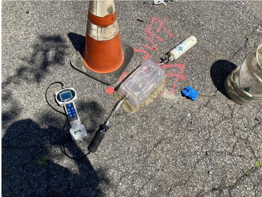
Photo 3: View of helium tracer test at SV-17
