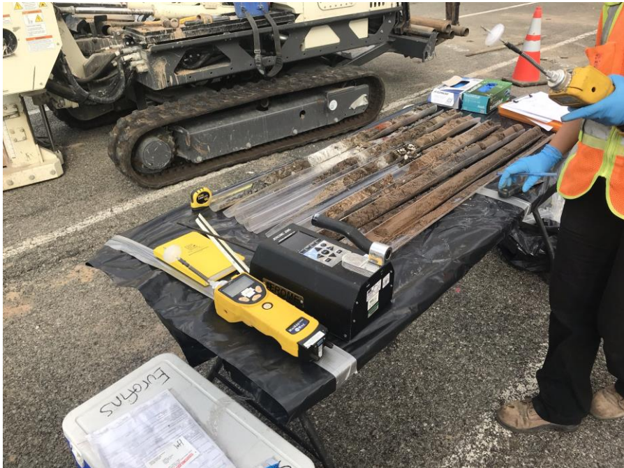
Photo 4: Langan preparing to screen soil for VOCs (facing northwest)
