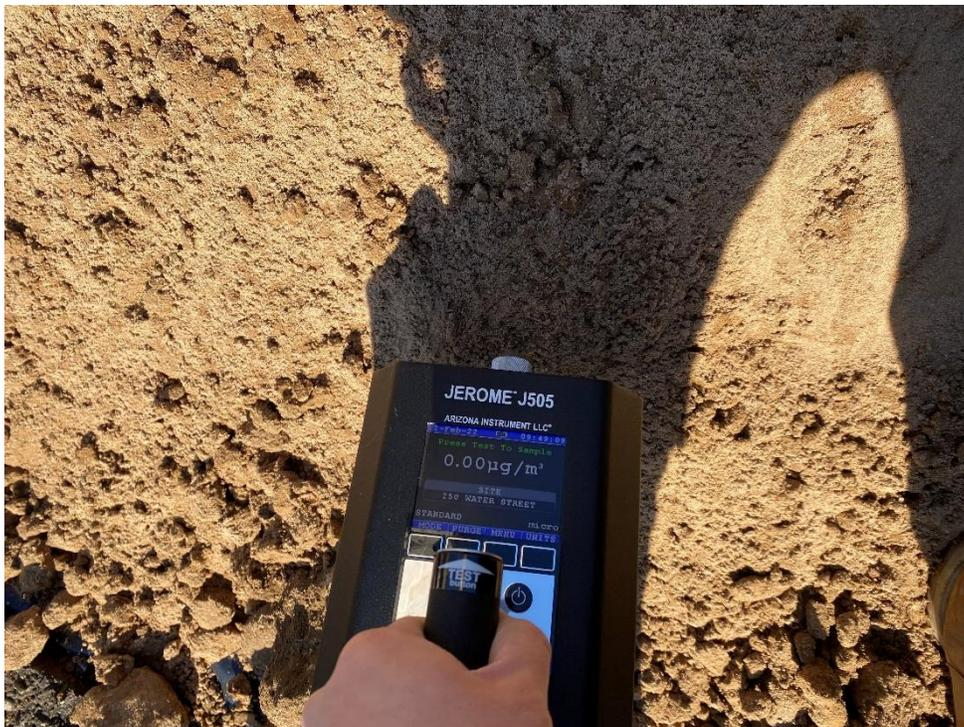
**Photo 4:** View of Langan screening excavated soil/fill from test pit TP01 using a Jerome® J505 mercury analyzer (02/12/2022)
