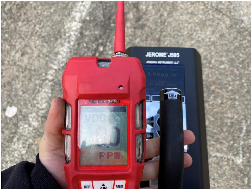
**Photo 13:** View of the RKI GX-6000 PID and Jerome® J505 used for work zone and ambient air screening (02/12/2022)
