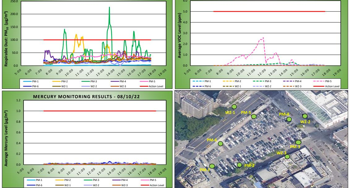
Air Monitoring Notes: Langan performed air monitoring at the perimeter of the site and at work zones at nine total locations for mercury vapor, volatile organic compounds (VOCs), and particulate matter less than 10 microns in diameter (PM10), during ground-intrusive activities. There were no fifteen-minute average concentrations for VOCs, and mercury vapor that approached or exceeded the action level established by the CAMP (5.0 ppm, and 1.00 µg/m3, respectively).
