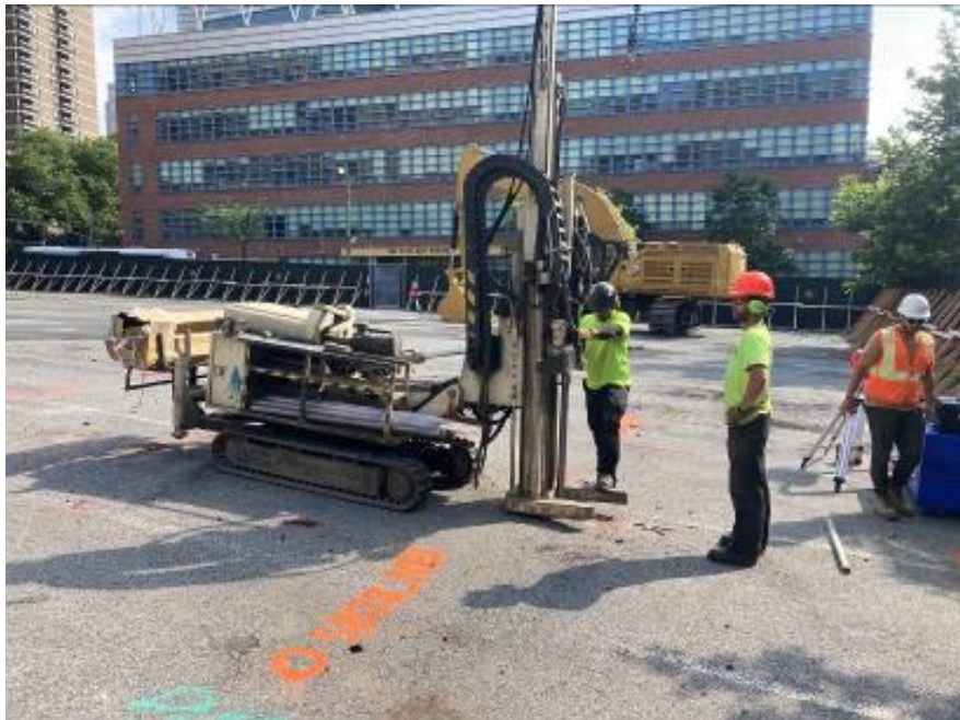
Photo 1: View of Lakewood advancing a soil boring in the south-central part of the site (facing east).
