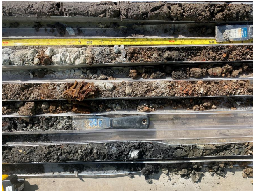
Photo 2: View of soil/fill recovered from waste characterization soil boring WC07A.
