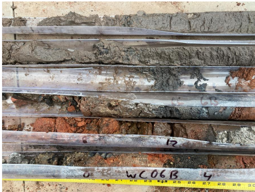
Photo 2: View of soil/fill recovered from waste characterization soil boring WC06B.
