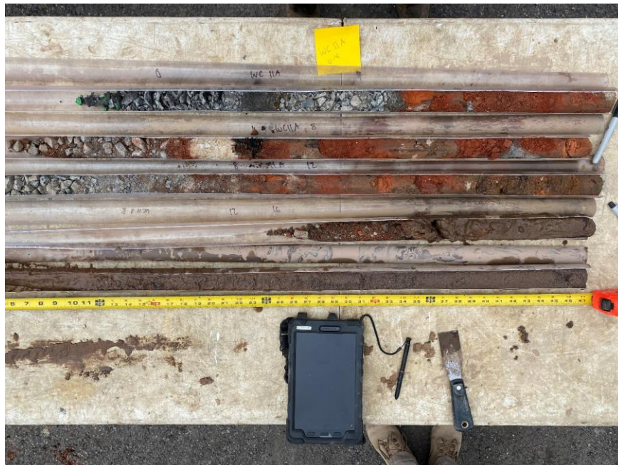
Photo 2: View of soil/fill recovered from waste characterization soil boring WC11A.
