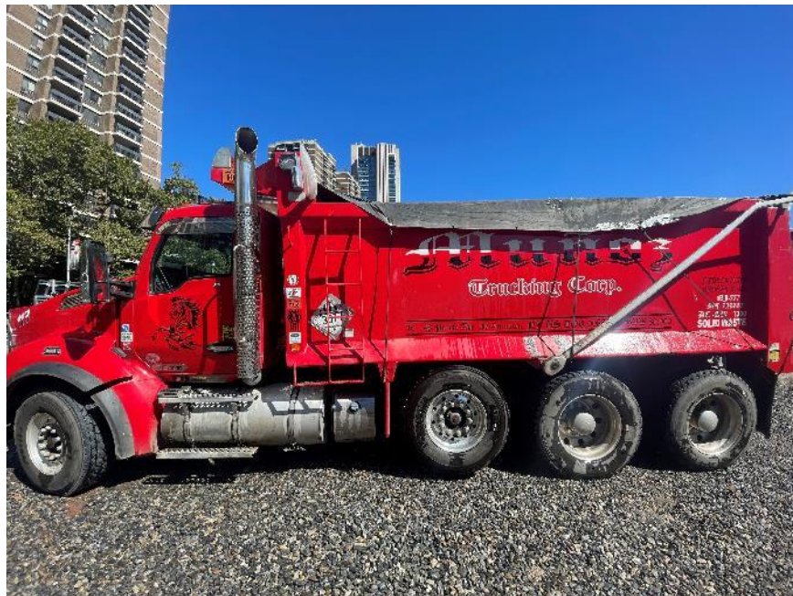
Photo 2: Tri-axle dump truck loaded with excavated soil/fill for off-site disposal, secured with a tight-fitting cover (facing east)
