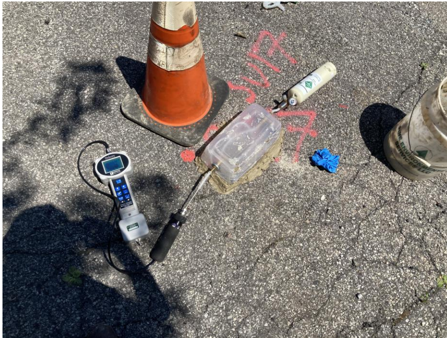
Photo 3: View of helium tracer test at SV-17
