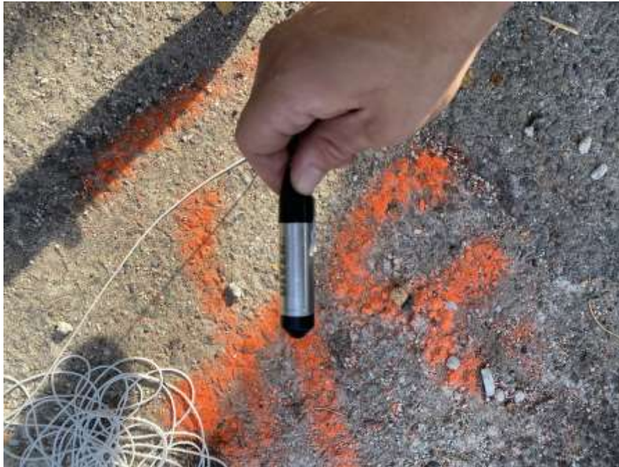
Photo 1: View of submersible datalogger
