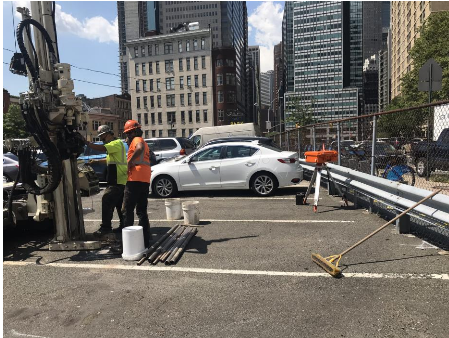
Photo 1: AARCO advancing soil boring SB24 in the northern part of the site (facing southwest)
