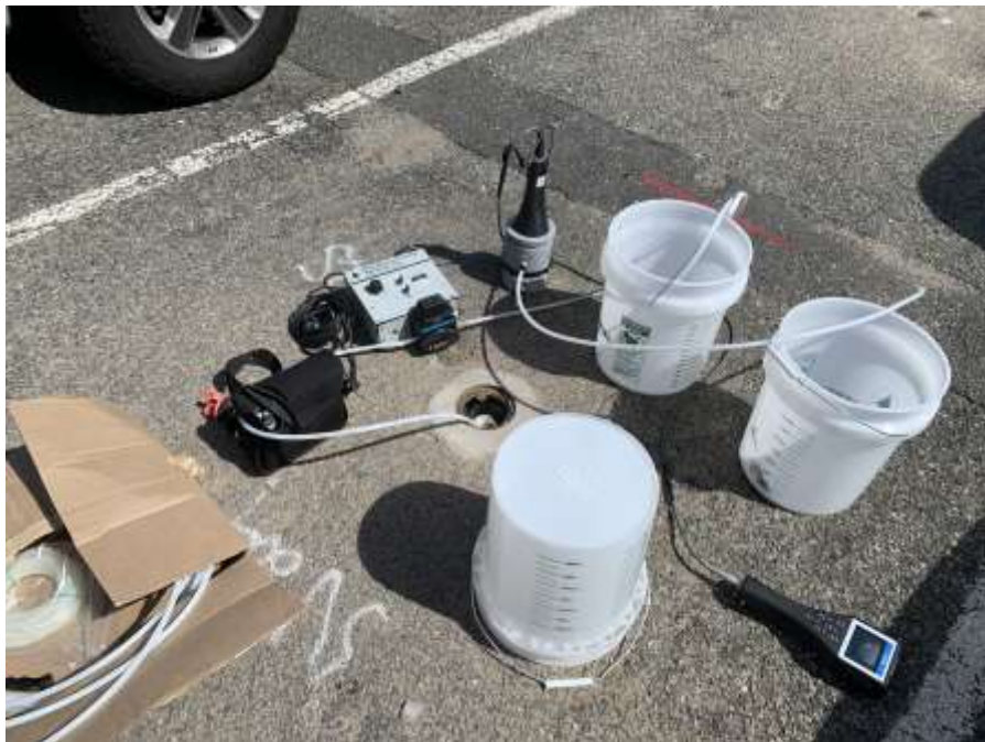
Photo 4: Typical groundwater sampling set up
