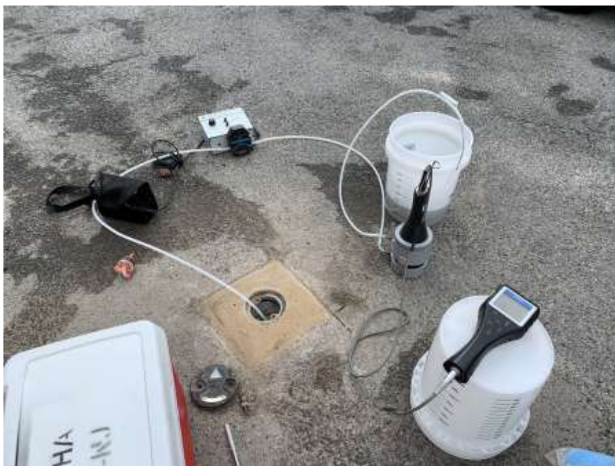
Photo 4: Typical groundwater sampling set up
