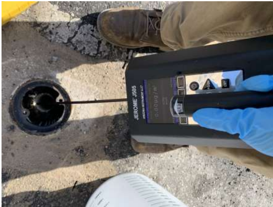
Photo 3: Typical Jerome screening at monitoring well
