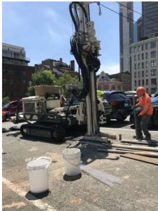
Photo 1: AARCO advancing soil boring SB4W1 (facing southwest)
