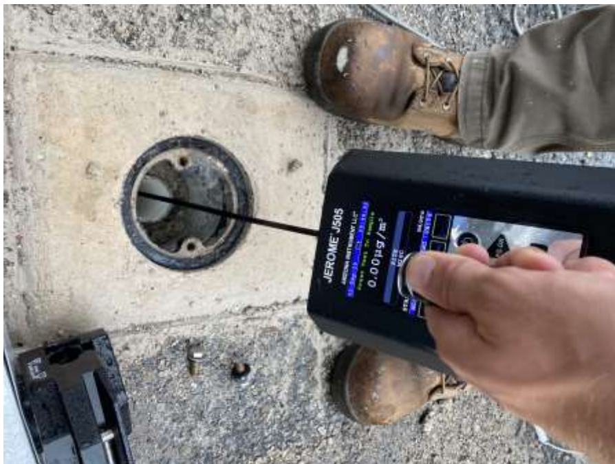
Photo 3: Jerome screening at monitoring well MW34
