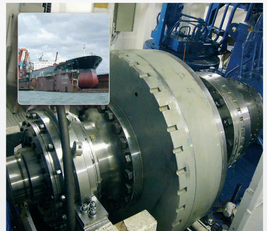
Engines, gearboxes and propeller shafts on ships are aligned using Easy-Laser® system. Thanks to versatile brackets you can install the equipment in the most appropriate place; shaft, coupling or flywheel.
