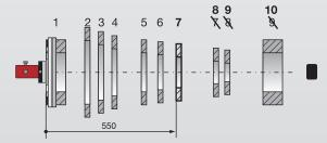
It's easy to add measurement points anywhere on the object in an existing measurement. The following points will be renumbered automatically. If you remove a point the following will be renumbered according to the same principle. If you remeasure a point, the old values will be saved in a history data base for possible later comparison. All this you can do at any time during the measurement!
