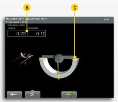
3. "Live" adjustment of the measurement object. Vertical and horizontal value for the object (B). Markings on the circle shows zone for adjustment with live values (C).
