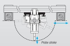
The measuring principle is the same for bracket A and B. The probe rod is very easily adapted to each diameter with extensions of different length (right). Bracket A has a stroke of 10 mm, B 60 mm.
