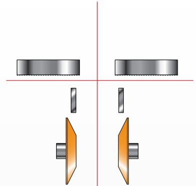
The laser beam (red) is pointed along the chain, representing the centre line to which the saw blades, reducers and steerings are aligned and positioned. Then the beam is angled 90°. All four band wheels (upper, lower, left, right) must be aligned to each other and to the centre line. The reducers are angled according to specifications.
