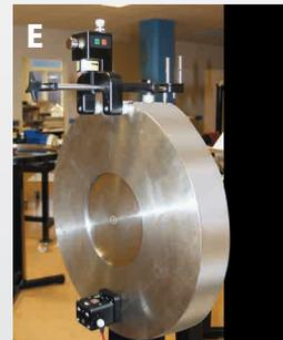
A. The rigid laser transmitter bracket allows for easy indexing (90°) to the band wheel. The wheels are aligned 90° to the centre line chain. The laser makes a constant sweep parallel to the wheel, which means you just place the detector anywhere within the laser sector and read off the value.
