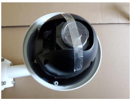
Remove the tape and lens cover and set aside for possible shipping, perhaps for warranty repair, should that be necessary.
