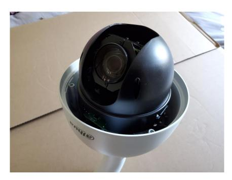
Replace the dome onto the camera, **taking care that the o-ring is in place** and tighten the three screws.
