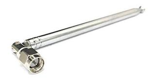
This is typically a ¼ wave whip which is omnidirectional but has no well-defined ground plane. Its gain at any particular frequency is dependent on its extended length. The optimal values may be calculated using this Whip Antenna Length and Frequency Calculator:
