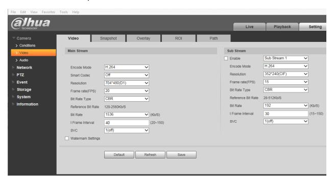
Above shows frame resolution for 704 x 480, 20 frames per second.
