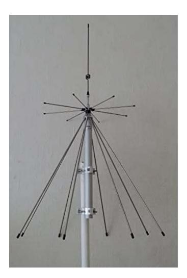
The horizontal and conical elements are the primary antenna and the vertical element extends it low-frequency response. Its response is omnidirectional, primarily in the horizontal plane.
