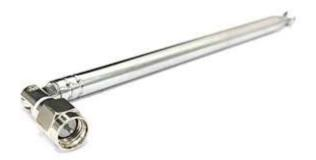
This is typically a ¼ wave whip which is omnidirectional but has no well-defined ground plane. Its gain at any particular frequency is dependent on its extended length. The optimal values may be calculated using this Whip Antenna Length and Frequency Calculator:
