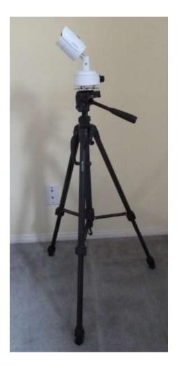
3. The initial height of the camera may be adjusted by spreading the tripod legs and by how far the legs are extended. To extend them, unlatch, extend/retract and re-latch. For stability, it is better to spread the legs to a wider rather than narrower stance and extend the legs if necessary to achieve a desired height.
