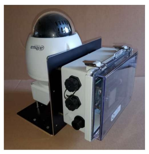
Any camera and the MSDAU are powered via their own Ethernet cable to PoE injector. In the above configuration, the camera and the MSDAU each require an Ethernet cable to an injector, usually located near a router.
