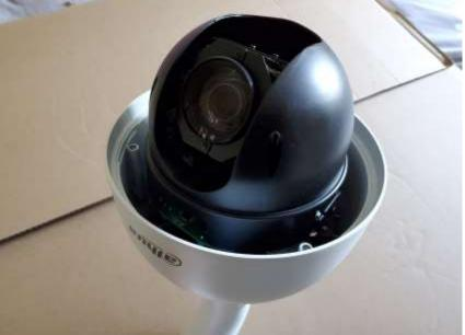
Replace the dome onto the camera, **taking care that the o-ring is in place** and tighten the three screws.
