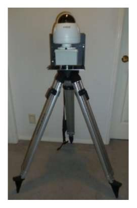
Note that the tripod legs may be extended and spread from vertical to fully horizontal to accommodate a wide range of height and stability requirements. However, if the legs are spread too far, then the leg tips cannot grip the ground which may result in undesired spread.
