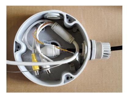
5. Reinstall the shroud to the nut and tighten the shroud by hand as much as possible. Be sure that the rubber gasket under the shroud has fully tightened against the cable.
