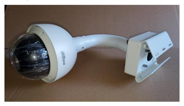
The junction box provides a waterproof transition from the camera's Ethernet connector to a box-mounted connector you use to attach the Ethernet cable.
