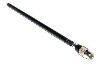
This is typically a ¼ wave whip which is omnidirectional but has no well-defined ground plane. Its gain at any particular frequency is dependent on its extended length. The optimal values may be calculated using this Whip Antenna Length and Frequency Calculator:
