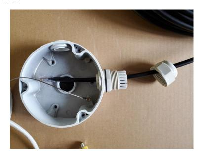
4. Plug the cable into the camera's Ethernet jack and dress the cables inside the box as shown:
