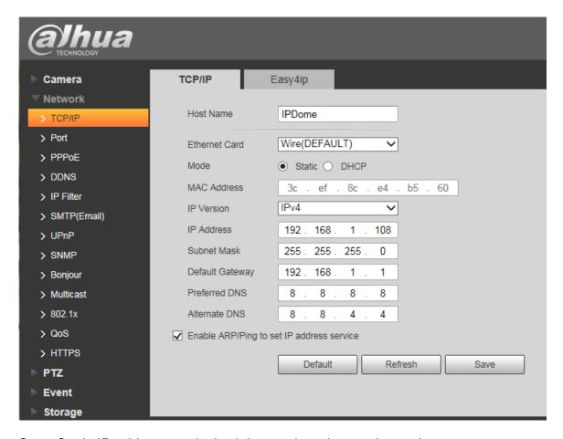
Set a Static IP address as desired. Leave the other setting as is.
