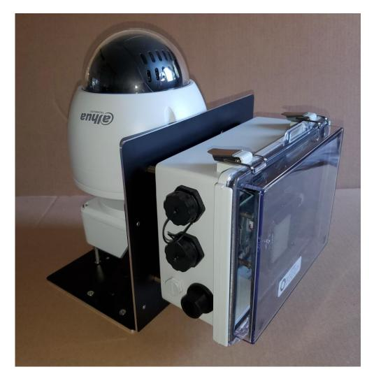
Any camera and the MSDAU are powered via their own Ethernet cable to PoE injector. In the above configuration, the camera and the MSDAU each require an Ethernet cable to an injector, usually located near a router.
