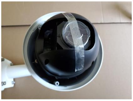
Remove the tape and lens cover and set aside for possible shipping, perhaps for warranty repair, should that be necessary.
