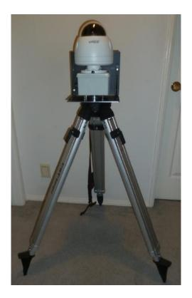
Note that the tripod legs may be extended and spread from vertical to fully horizontal to accommodate a wide range of height and stability requirements. However, if the legs are spread too far, then the leg tips cannot grip the ground which may result in undesired spread.
