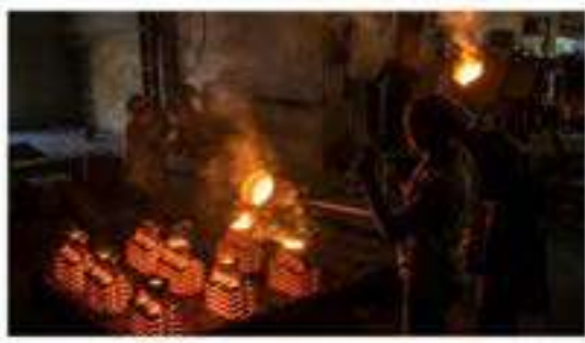
MELTING DEPARTMENT OF FOUNDRY - 4 AIR-MELT FURNACES - 100kgs, 150kgs, 300kgs, 500 kgs
