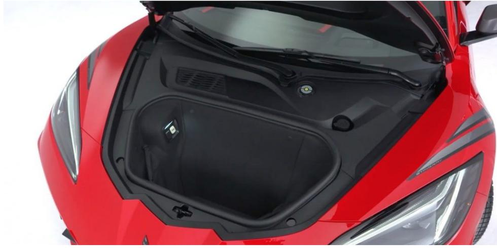
As Corvette chief engineer Tadge Juechter explains in the informative video embedded below, some 2020 Corvette owners were accidentally hitting the front trunk pop on their key fob and unlocking the hood before setting off on their journey. With the vehicle's speed [limited to 82 mph with the front trunk open](#), some owners reached a high enough speed to cause the panel to [open violently and in some cases damage the hinges](#) and front fenders and scratch the paint.
