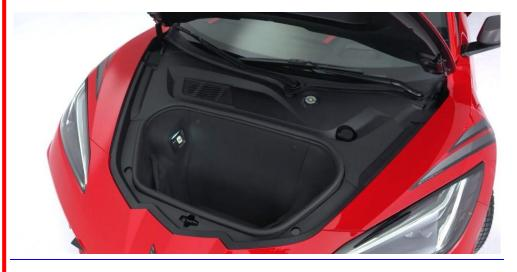
As Corvette chief engineer Tadge Juechter explains in the informative video embedded below, some 2020 Corvette owners were accidentally hitting the front trunk pop on their key fob and unlocking the hood before setting off on their journey. With the vehicle's speed <u>limited to</u> <u>82 mph with the front trunk open</u>, some owners reached a high enough speed to cause the panel to <u>open violently and in some cases damage the hinges</u> and front fenders and scratch the paint.
