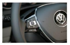
Adaptive cruise control (ACC) is an available cruise control system for road vehicles that automatically adjusts the vehicle speed to maintain a safe distance from vehicles ahead.
