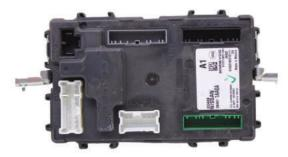
Do the lights or wipers no longer work? Then there may be problems with the **Body Control Unit. BCM controls** components such as: lights, windows, door locks and various comfort controls.
