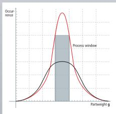
Logging of highly variable input signals with high temporal resolution enables precise control of the injection molding process. As a result, the working window becomes narrower, and part weight fluctuations and material consumption are reduced.
