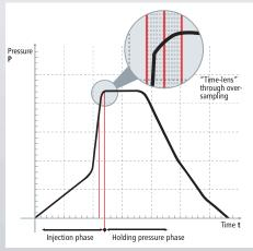
XFC enables high-resolution analysis of the corresponding pressure curve. Oversampling enables resolutions even below the minimum I/O response time. The distributed synchronised clocks, combined with the time stamp functionality of EtherCAT, facilitate sampling at precisely defined times.
