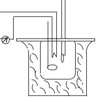
The beaker contains kerosene oil. A resistor is kept submerged into the beaker. The terminals of the resistor is kept connected to a e.m.f. source having a variable resistor along with an ammeter.
