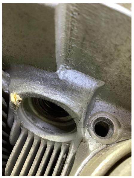
Note in the picture what appears to be a crack between the intake port and the smaller fuel injection port. The roughly horizontal crack runs across the roughly vertical web between the two ports. This type of crack is often caused by over tightening the fuel injector.
