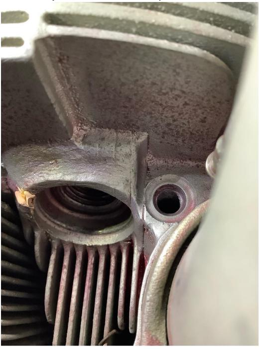
So, what caused the original issue of an apparent crack on the cylinder. I don't know for sure, but it appears to have been just dirt and/or grease smeared in a line. The line was in an area where cracks can occur, so it was easy to assume a crack. Based on the article by Mike Busch it may be an issue on Cirrus aircraft. Something in the cowling/baffling may cause an airflow that deposits the dirt/stain in a location and orientation that looks like a crack.
