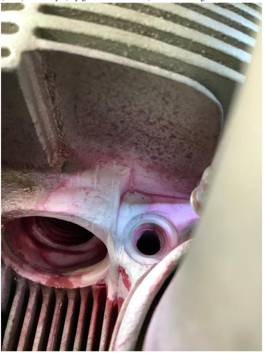
In this case it is obvious there is no dye color in the area of the suspected crack. The cylinder head was not cracked! I could hear the owner sigh in relief a block away. As a bit of a quality control, note the area just below the injector port in the face of the cylinder where there is a red reaction area. This appears to be a porous spot in the casting. It is not a structural issue, but being there, shows up in the process, indicating we probably did it right.
