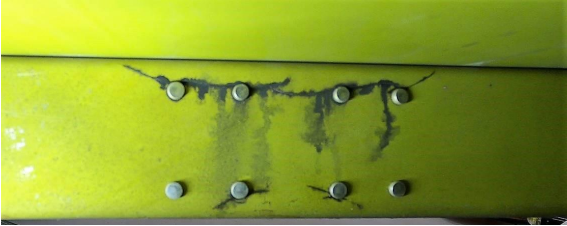
FIGURE 2: EXAMPLE 1 - CRACK LOCATIONS - FWD SIDE OF SPAR
