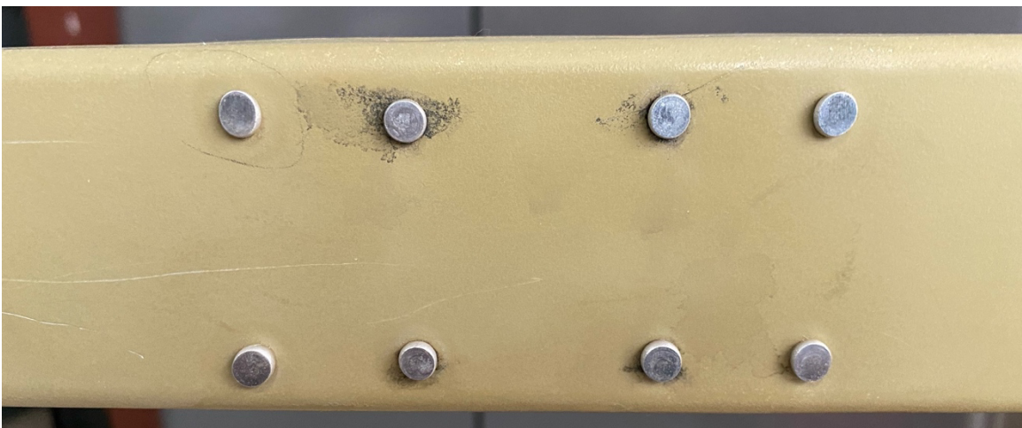
FIGURE 3 - EXAMPLE 2 - CRACK LOCATIONS - FWD SIDE OF SPAR
