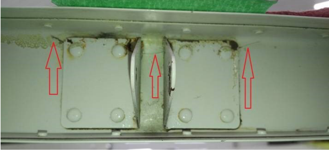
FIGURE 1 – EXAMPLE 1 - CRACK LOCATIONS – AFT SIDE OF SPAR
