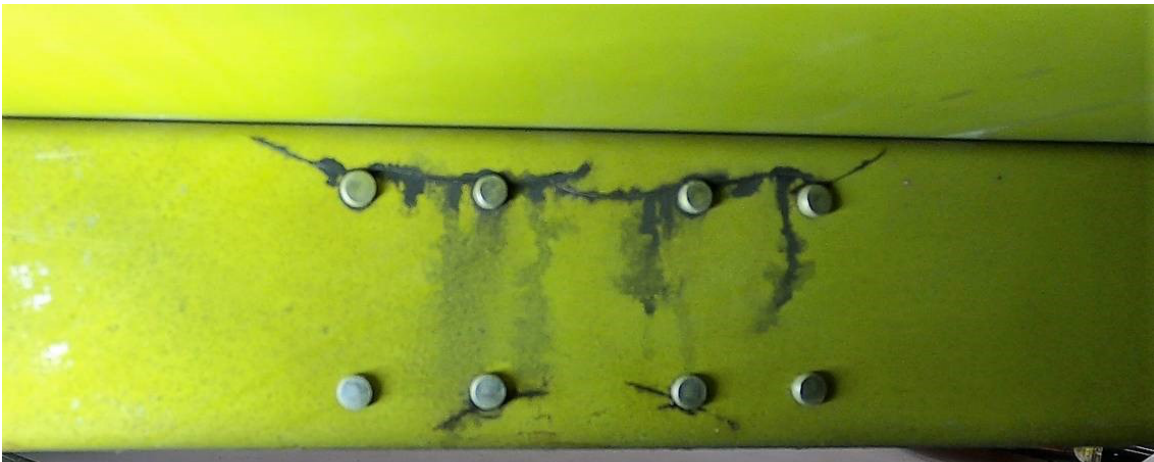
FIGURE 2 - EXAMPLE 1 - CRACK LOCATIONS - FWD SIDE OF SPAR
