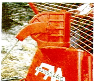
The upper pulley - very strong, load-shock proof.
