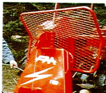
The lower pulley is well situated for stability and sidepulling.
