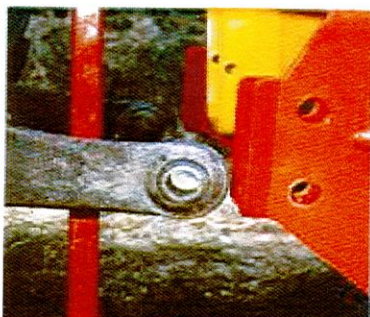
Simple 3 point linkage mounting.
