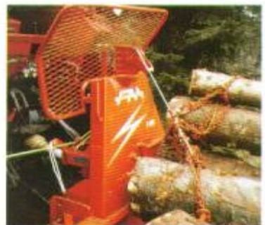
Sufficient height of the winch allows a lot of ground clearance for the timber.
