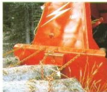
Robust hill support plate with a wide log-towing bar.
