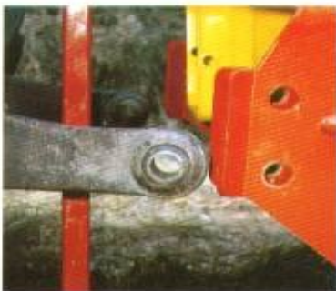
Simple 3 point linkage mounting.
