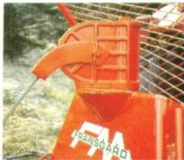
The upper pulley - very strong, load-shock proof.
