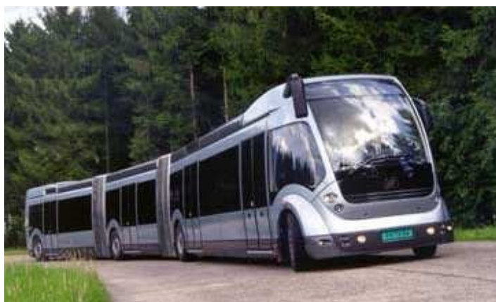
Figure 7.1.3 Advanced Public Transport Systems (APTS), Phileas bi-articulated bus with hybrid engine, operated in Netherlands and France. Capacity 185 passengers. (APTS, 2008).
