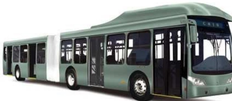
Figure 7.1.2 Caio Induscar, Mondego LA articulated bus, operated in Santiago, Chile. Capacity 160 passengers (Caio, 2008).
