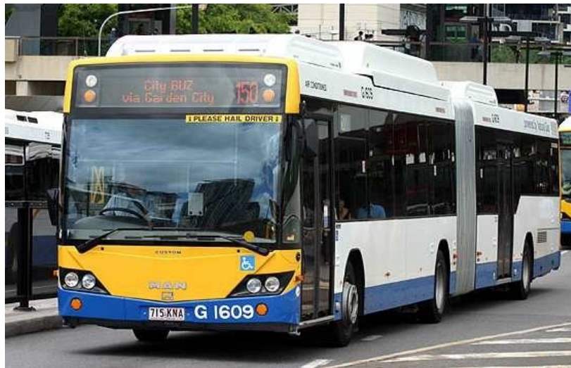
Figure 7.1.1 Man NG313 articulated bus, operated by Brisbane City Council. Capacity 85 passengers (BTBuses, 2008)
