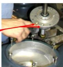
Align Grease Fill & Relief Ports on the bearing carrier, align with the grease zerk (fill port) on the housing.
