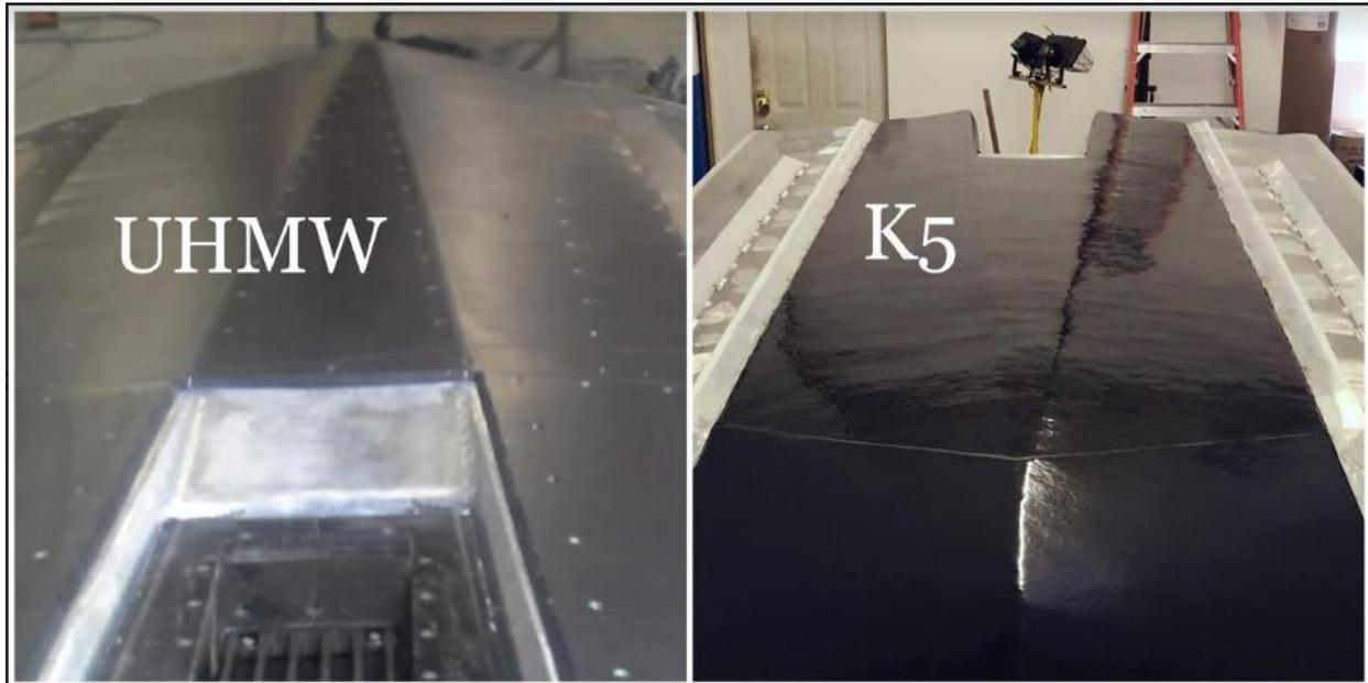
As a final step to putting my money where my mouth is, I am taking a hull that had UHMW on it and testing it for a year with K5. This is a 3/16" Hull with 4'x15' section of 1/4" aluminum welded to it. A true heavy duty hull coated with K5 and Wetlander. Need to thank the folks at Premium Protective Coatings for assisting me in this test.
