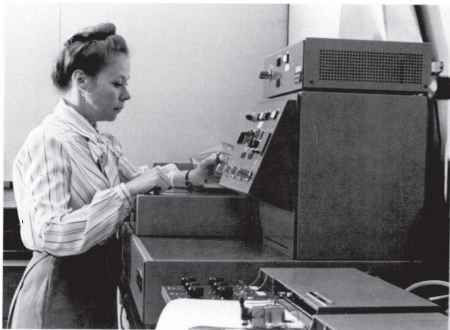
Fig. 3. The thermal analysis lab uses differential scanning calorimetry (DSC), thermogravimetric analysis (TGA), and thermomechanical analysis (TMA) to determine such parameters as melting point, heat capacity, glass transition temperature, expansion coefficients; and to monitor such phenomena as thermal degradation of polymers.
