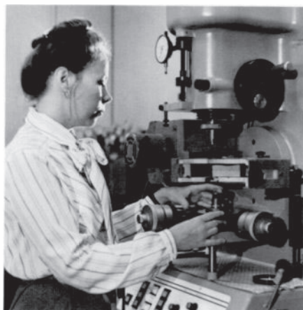
Fig. 4. The Rheometrics mechanical spectrometer is a versatile device that can subject the test sample to a variety of static and time-varying stresses at different temperatures, while monitoring mechanical response. Dynamic viscosity and elastic modulus are two parameters that can be measured.
