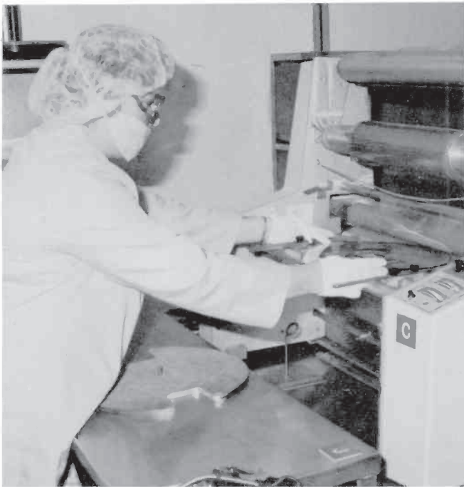
Fig. 7. Coating application. The stampers that must be handled through finishing operations have the front face protected by application of a protective plastic film.
