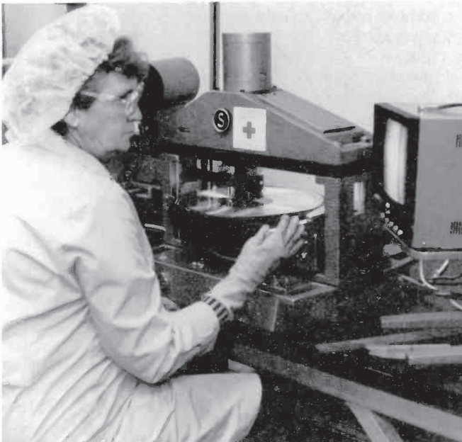
Fig. 9. Centering operation. The stamper concentricity is established by a centerhole punch using a video camera focused on a "recorded-in" centering ring.
