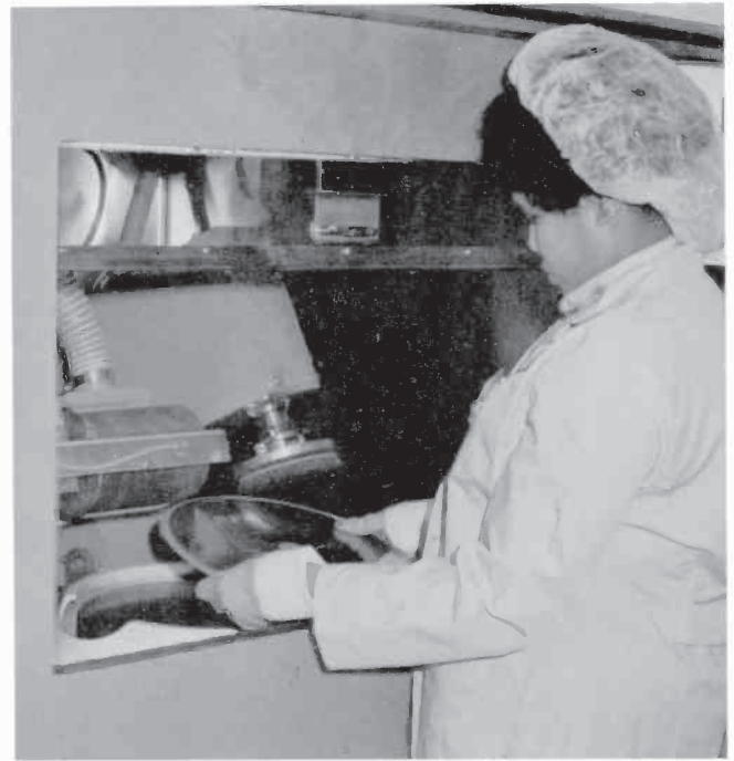
Fig. 8. Stamper backfinishing. The stamper backs are ground and polished to a smooth surface in an automatic finishing machine.
