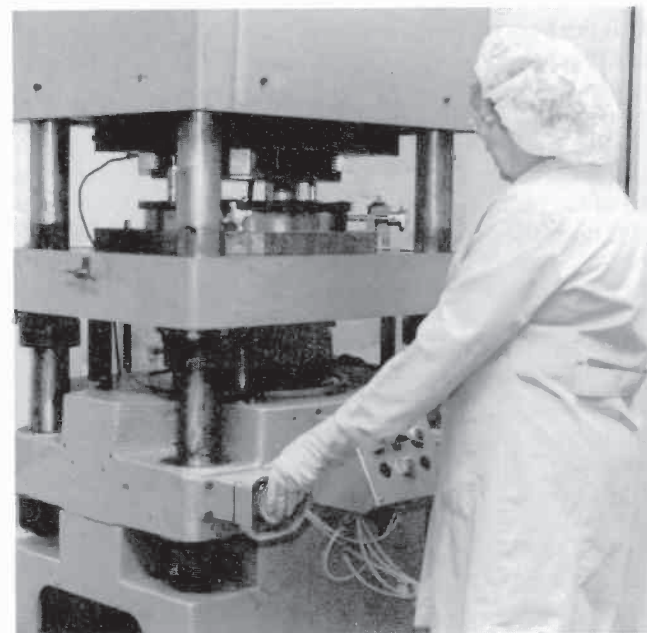
Fig. 10. Coining die. The mechanical profile of the inner and outer edges of the stamper is formed in a coining operation. The forming allows a match between the stamper and the press-mold geometries.
