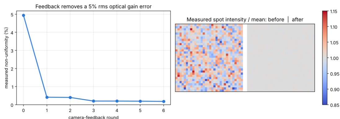
Camera feedback: measured non-uniformity per round (left) and the spot map before and after (right).
