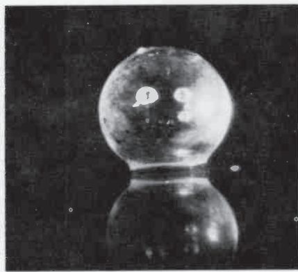
Fig. 4. A glass ball, 2.5 mm in diameter, rests on a glass substrate. A sodium carbonate particle, mass 300 times less than the ball, lies next to the ball. In (a), the humidity is below 78 percent and the particle is dry. In (b), the humidity has been raised to 90 percent and the sodium carbonate is
