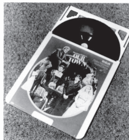
Fig. 3. VideoDisc caddy. Because of the very small dimensions of the recorded information, the disc is kept in a protective plastic sleeve, or caddy, at all times except when being played in a player. The plastic frame surrounding the disc, called a spine, serves to move the disc into and out of the protective sleeve when the disc is inserted into and retrieved from a player.
