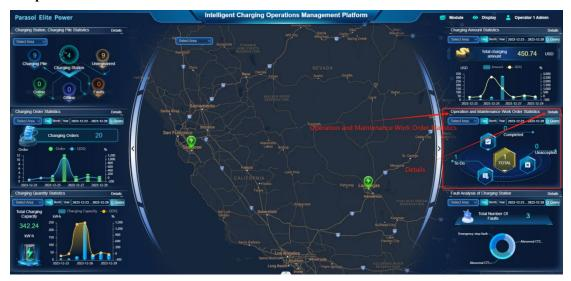
Tabulate the total number of operation and maintenance work orders, completed, pending, and outstanding quantities within the specified time range. Click on "Details" to access statistical details regarding the operation and maintenance work orders.
