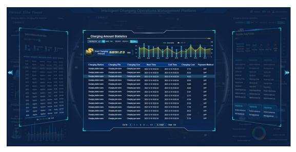
Compute the total charging amount based on the operating area, charging station, time range, and other specified conditions. Display the daily, monthly, and annual charging amounts through a graphical representation. For detailed insights into each charging amount, including charging station, charging pile, charging gun, charging start time, charging end time, charging fee, and payment method, refer to the details section.
