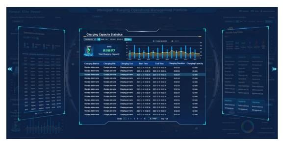
Compute the total charging capacity based on the operating area, charging station, time range, and other specified conditions. Present the daily, monthly, and annual charging capacity through a graphical representation. For detailed insights into each charging session, including charging station, charging pile, charging gun, charging start time, charging end time, charging duration, and charging level, refer to the details section.
