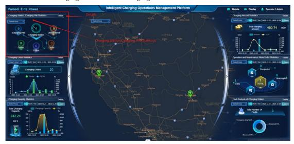
Count the number of charging stations and charging piles, including both online and offline quantities, fault occurrences, and unregistered units. Access detailed statistics on charging stations and charging piles by clicking on the "Details" option.
