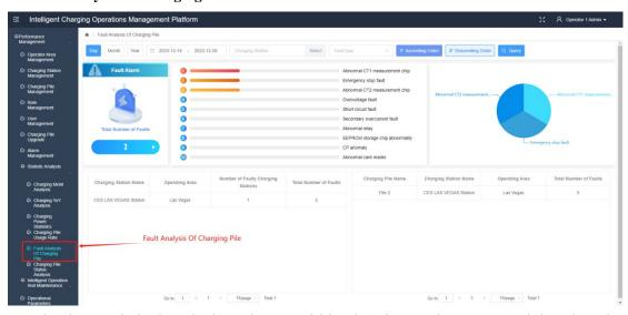
Conducting statistical analysis on issues within charging stations, categorizing them by fault type, charging station, and charging pile. Additionally, evaluating the distribution of different fault types.
