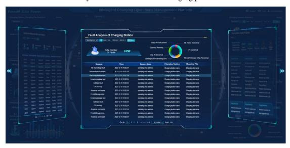
Calculate the total number of faults in charging stations, categorizing them based on operating areas, charging stations, time ranges, and other specified conditions. Analyze and present the proportion of various fault causes in a pie chart. For detailed information on each fault, including the cause of the fault, time of occurrence, charging station name, charging pile name, and other relevant details, refer to the details section.
