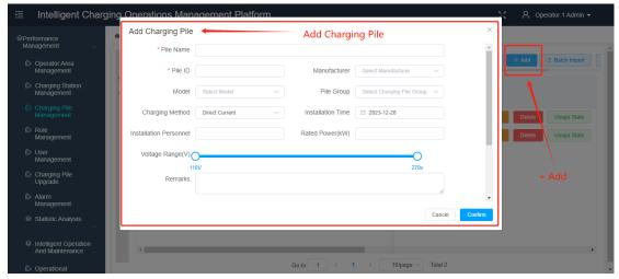
Click on "+Add" to open the new charging pile page and input the necessary charging pile information.
