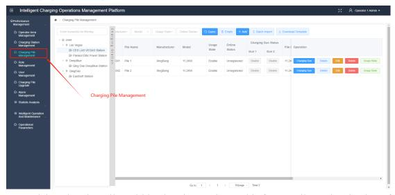
Supervising charging piles within charging stations. This feature allows the viewing of charging pile information organized by operational areas and charging stations. It supports the bulk import of charging pile details and enables the management of charging gun information for each charging pile.
