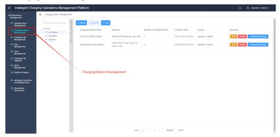
Supervising charging station information, facilitating the establishment of charging stations within operational areas, and configuring map coordinates for each station. Customers can utilize the app's charging navigation feature to easily discover stations and navigate to them.
