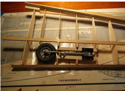
**Retract test-fitted into
