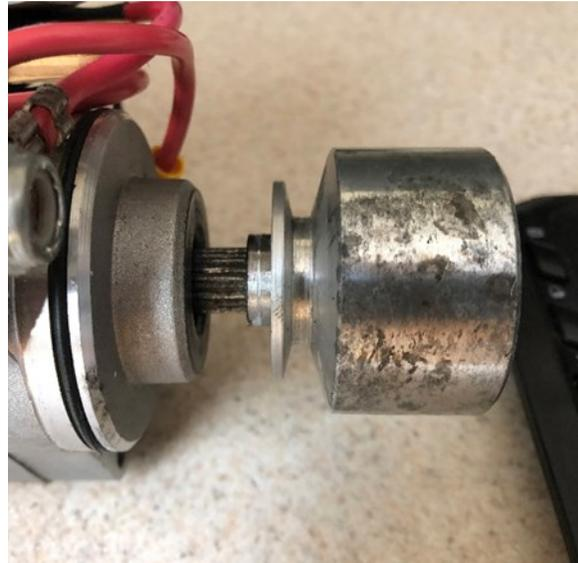
Above is the starter hub with sprocket pressed in. Note the sprocket is proud of the hub to prevent the starter hub from rubbing against the motor housing. I advise using JB weld or a set screw to secure the sprocket to the starter hub and keep it from slipping.
