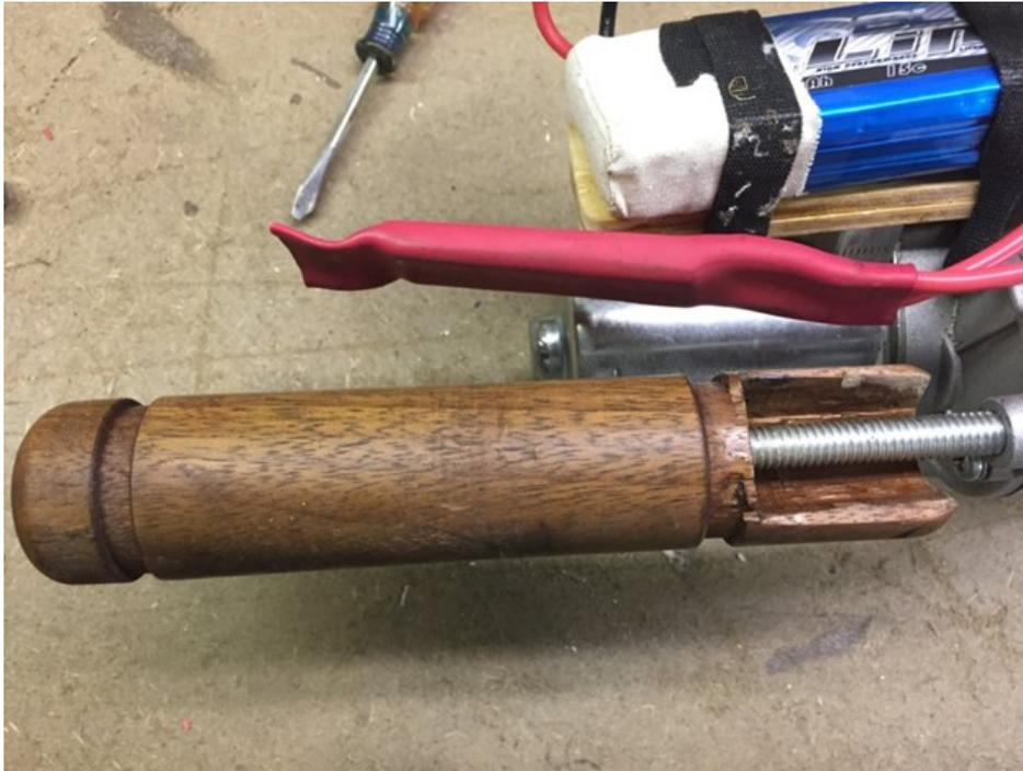
Here is the handle slipped over the threaded rod. Nut both ends to hold it in place.
