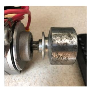
Above is the starter hub with sprocket pressed in. Note the sprocket is proud of the hub to prevent the starter hub from rubbing against the motor housing. I advise using JB weld or a set screw to secure the sprocket to the starter hub and keep it from slipping.
