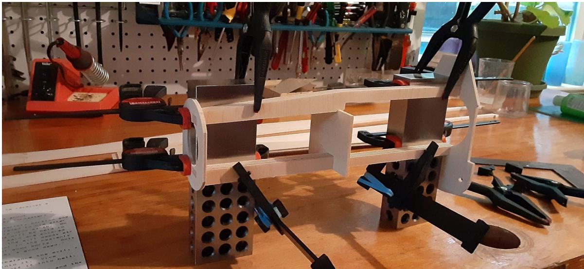
**An example of using four 1-2-3 blocks in constructing “The Cage” by the author**
