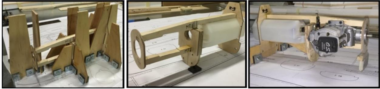
**An example of using a magnetic building board in the construction of “The Cage” by Duane Wilson with tank and engine**
