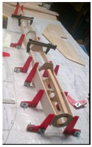
Use of a magnetic building board in building the fuselage in space by Bernie Olson
