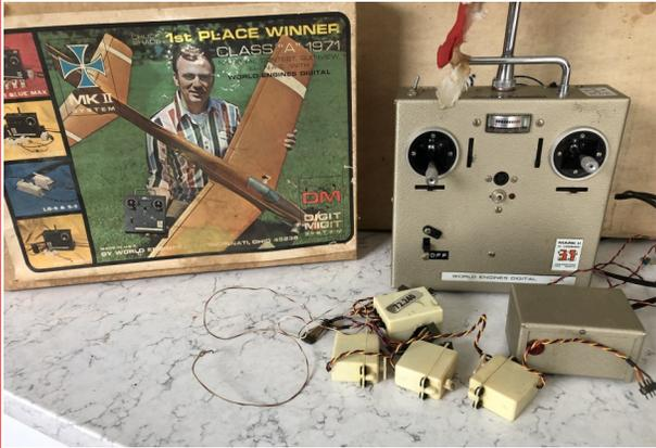
Finally in 1972, after lots of saving I got my first radio—a World Engines Blue Max MKII 6 channel radio set which I still have today. This was like a Heath Kit and you actually had to assemble it including soldering all the components and wiring.
