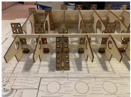
Magnets at the base of each rib guide grips to the metal sheet beneath the plans. Ribs are held in perfect 90° alignment for gluing.
