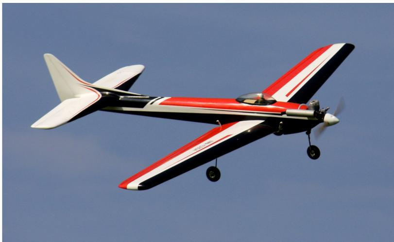
The raked vertical fin and rudder line was common to nearly all pattern planes from the
